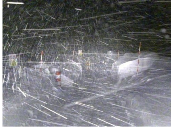
Fig. 8: RGB camera information in heavy snowfall environments
