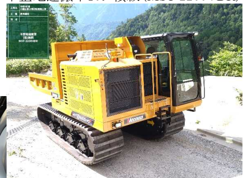
不整地運搬車10t 積級 (MST-2200VDR)
